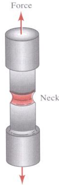
FIGURE 6-4 Localized deformation of a ductile material during a tensile test produces a necked region.
